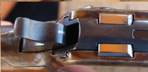
Notice the double locking lugs on the bolt to ensure a secure lock up identical to the 1886.
